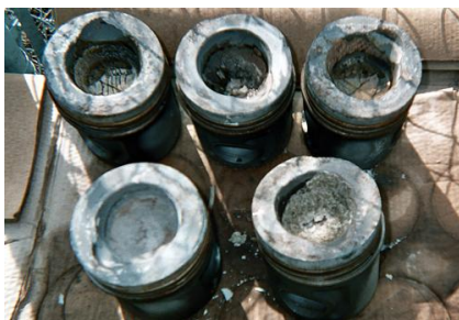
Siloxane deposits on engine pistons
