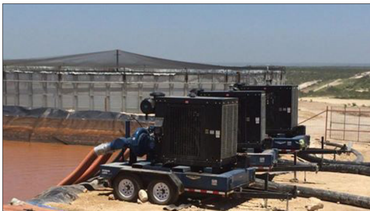
Pumps assist in moving water through above-ground and buried pipelines.
