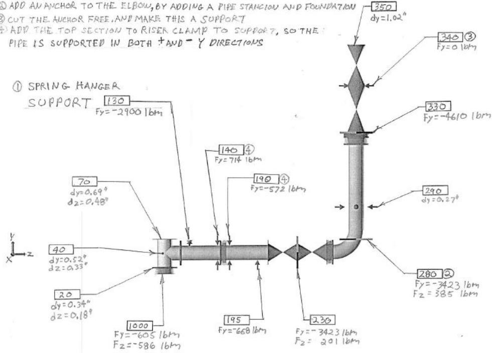
Figure 2: Analysis of an engine exhaust system under hot conditions.
